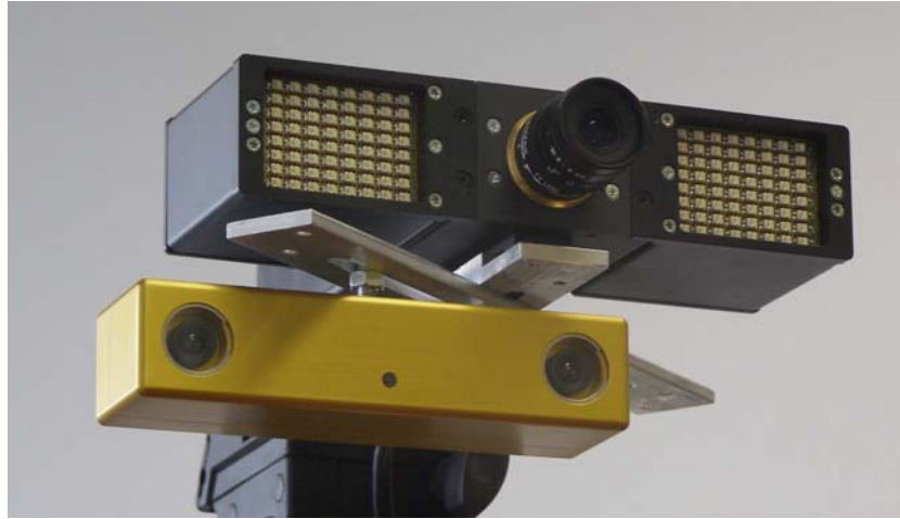
Fig. 1. All three cameras mounted on an aluminum bar
